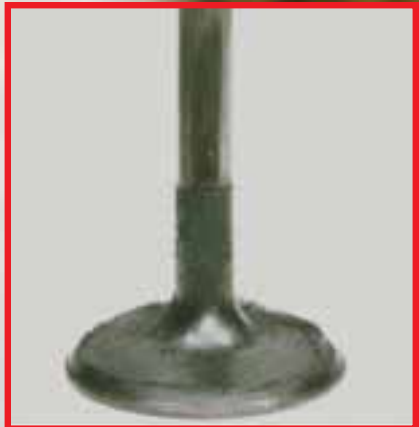
Intake valve after P.i. treatment
