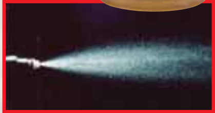
Injector spray pattern after P.i. treatment
